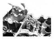
· Remove the oil jet (for oil spray) from the upper crankcase.
