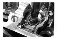
Insert the valves, with their stems coated with molybdenum oil solution all around and along the full stem length without any break.
