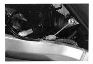
· Remove the fuel tank bracket mounting bolts.
