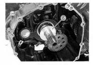
• Remove the thrust washer 1.
