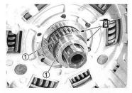
· Install the primary driven gear assembly.
