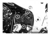
Remove the clutch release cylinder from the engine sprocket cover.
