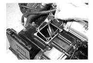
• Install the breather cover ① and the oil catch tank ② as shown.
