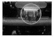
Disconnect the respective vacuum hoses from each throttle body.
